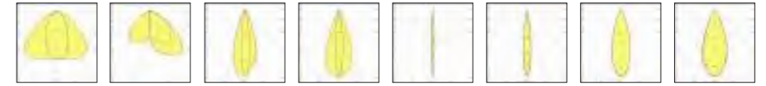
.RD Road .AS Asymmetric .VE Vertical Elliptical .HE Horizontal Elliptical .SS Super Spot .SP Spot .MD Medium .FL Flood
