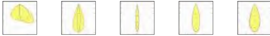
.WW Wall Washer .HE Horizontal Elliptical .SP Spot .MD Medium .FL Flood
